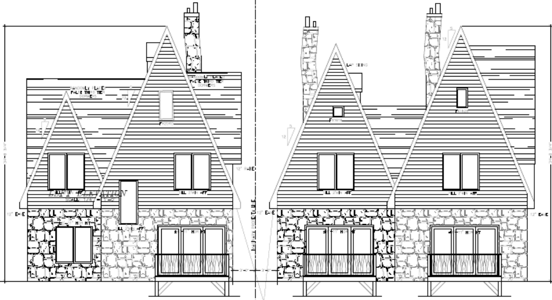
SOUTH ELEVATION (SOUTH SIDE UNITS) SCALE 1/4" = 1'-0"
