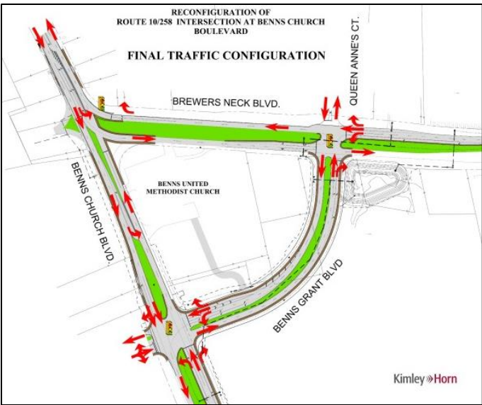
FIGURE 4 – RECONFIGURED BENNS CHURCH BLVD/ BREWERS NECK BLVD INTERSECTION
