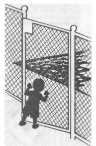
Where the release mechanism of the self-latching device is <u>less than</u> 54 inches from the bottom of the gate, the release mechanism for the gate shall be located on the pool side of the gate and be at least 3 inches below the top of the gate on the side facing the pool. Placing the release mechanism at this
