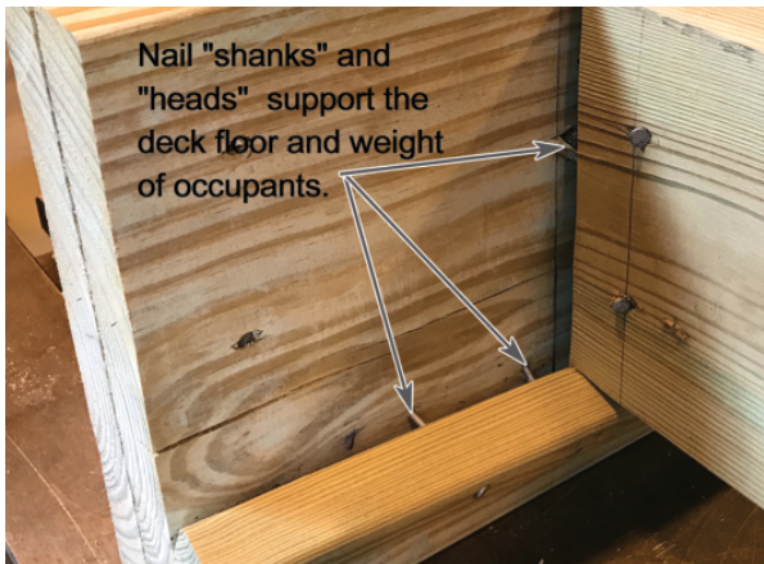
Photo 2. A test specimen after the test load was removed. The entire simulated occupant load was supported by the nail shanks and heads. For actual decks with this detail, occupants are supported in the same way.
