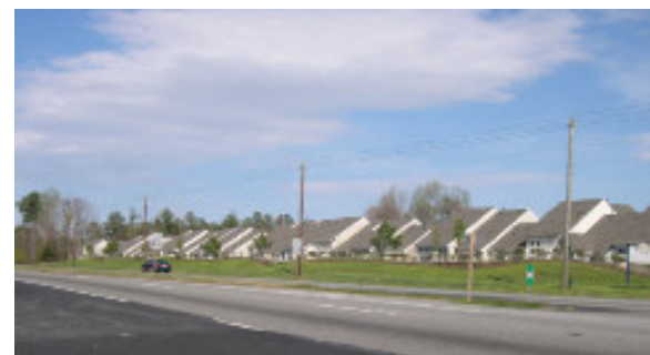
Inappropriate use of berming to limit views creates unnatural landscape appearance and does not adequately screen buildings
