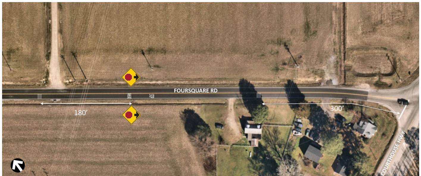
Figure 19. Overview of transverse rumble strip placement on Foursquare Road approach.
