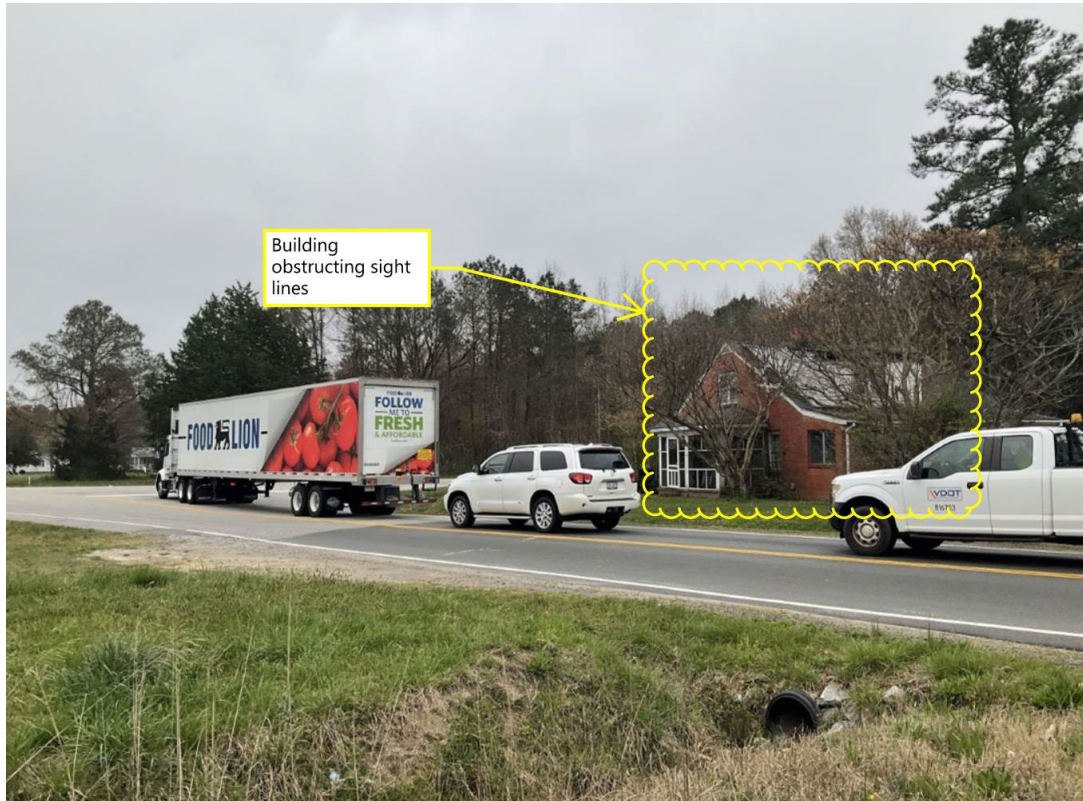
Figure 10. Building obstructing sight lines between turning vehicles on Foursquare Road and Courthouse Highway
