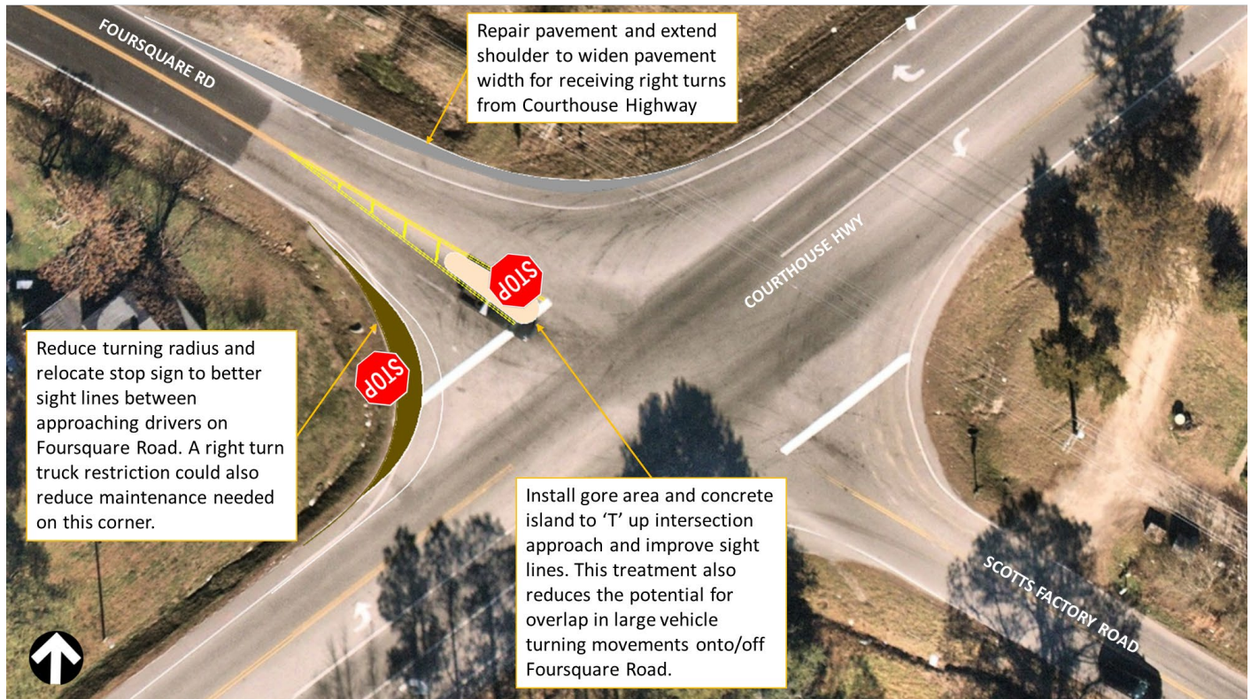
Figure 15. High-level concept showing stop sign visibility improvements
