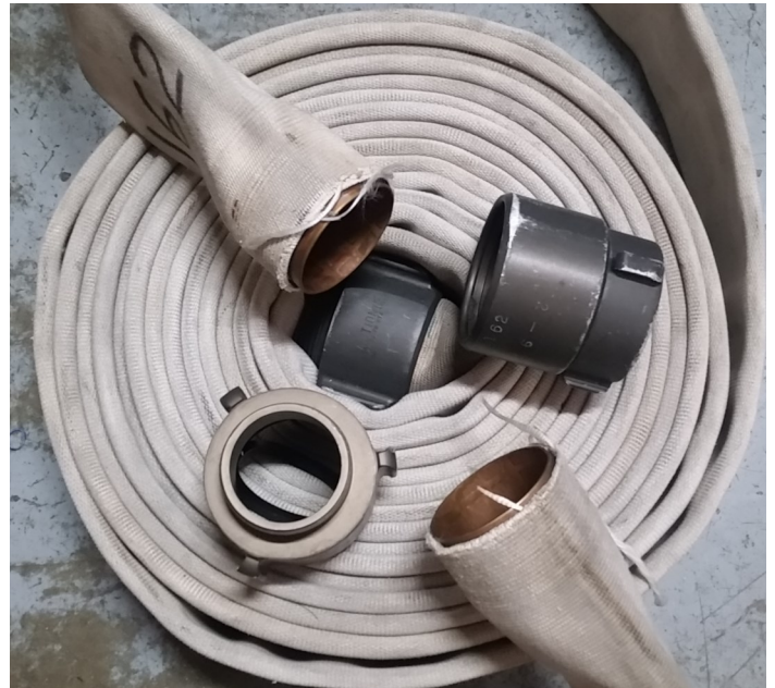
Tested fire hose with couplings that failed. Hose will be repaired and retested before putting back into service.
