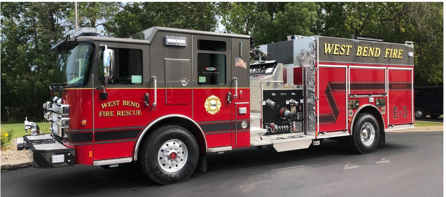
West Bend's newest fire apparatus was placed into service at the end of September. The 2019 Pierce Enforcer contains a 1,250 gallon per minute pump, a 1,000 gallon water tank, foam capabilities, ground ladders and enough storage to carry all the equipment required to be on a First Class Pumper. The vehicle is designed to safely carry a crew of four. Crews are finishing training and the engine will be stationed at Station #3. It is replacing a 20 year old vehicle that will be sold.
