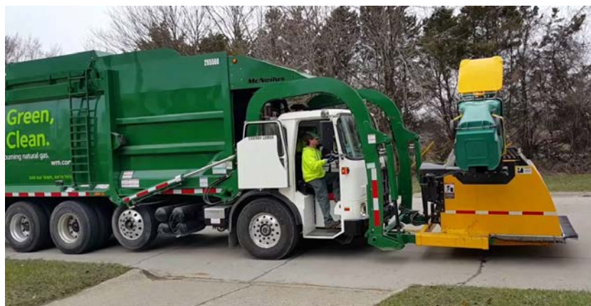
A WM truck equipped with the Curotto-Can system.
