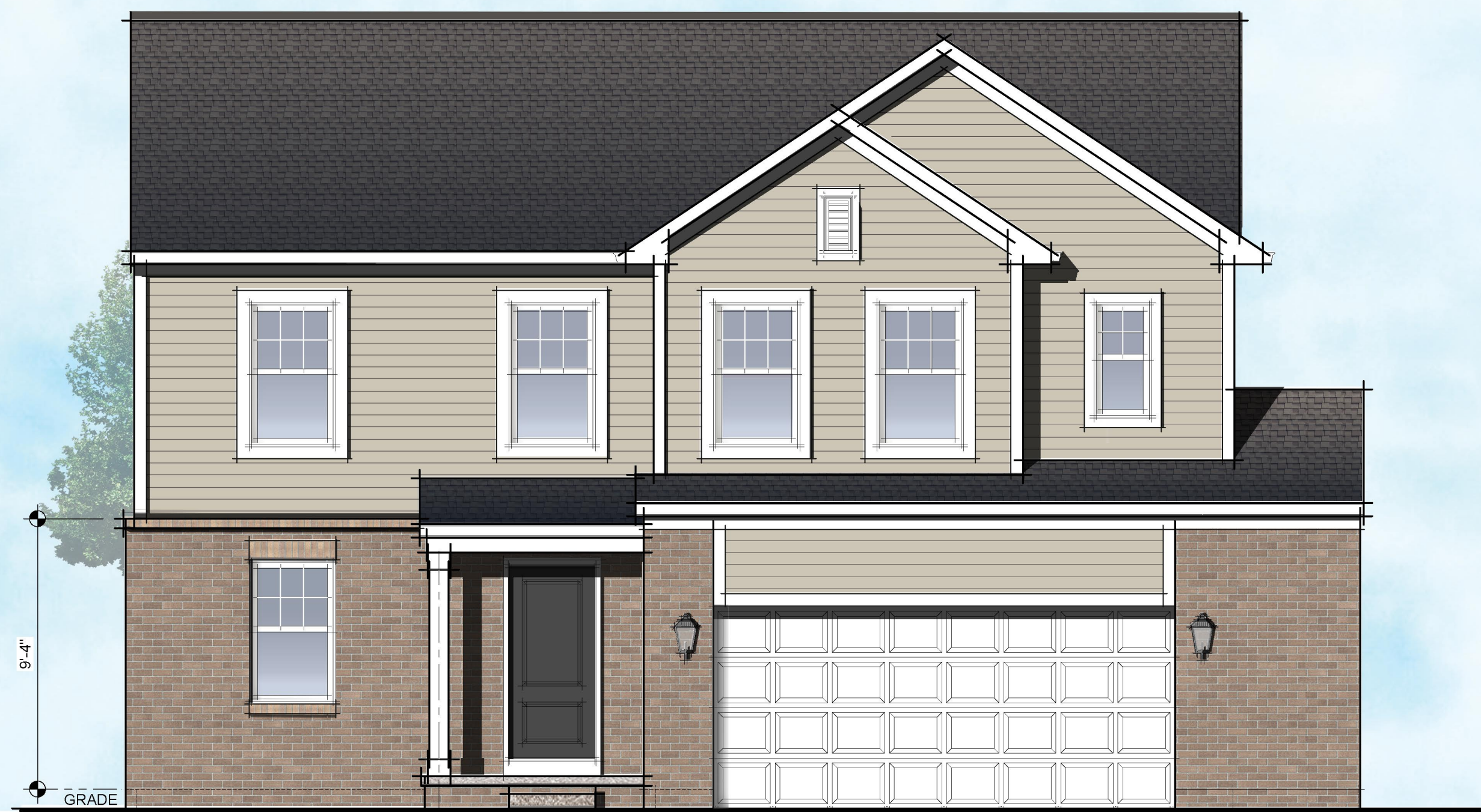
51.7% TOTAL MASONRY FRONT ELEVATION - E ESSENTIAL SERIES 6 SCALE: 1/4" = 1'-0"
