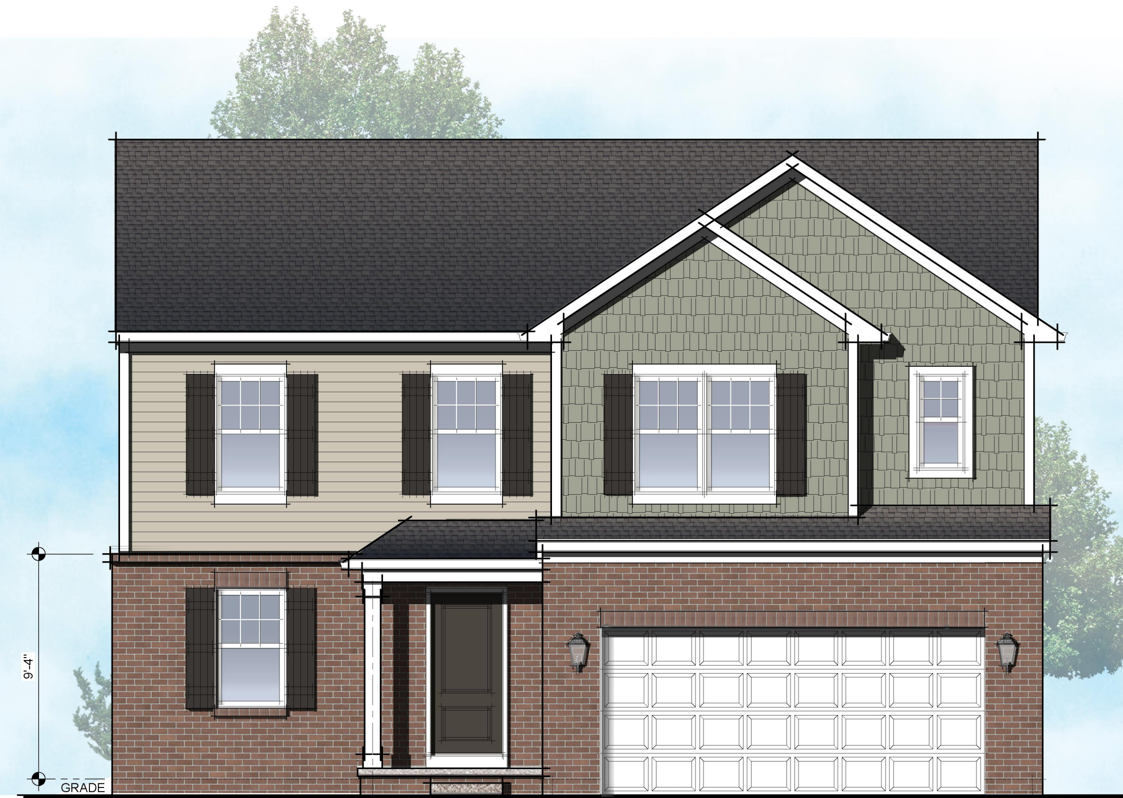
52.0% TOTAL MASONRY FRONT ELEVATION - F ESSENTIAL SERIES 3 SCALE: 1/4" = 1'-0"
