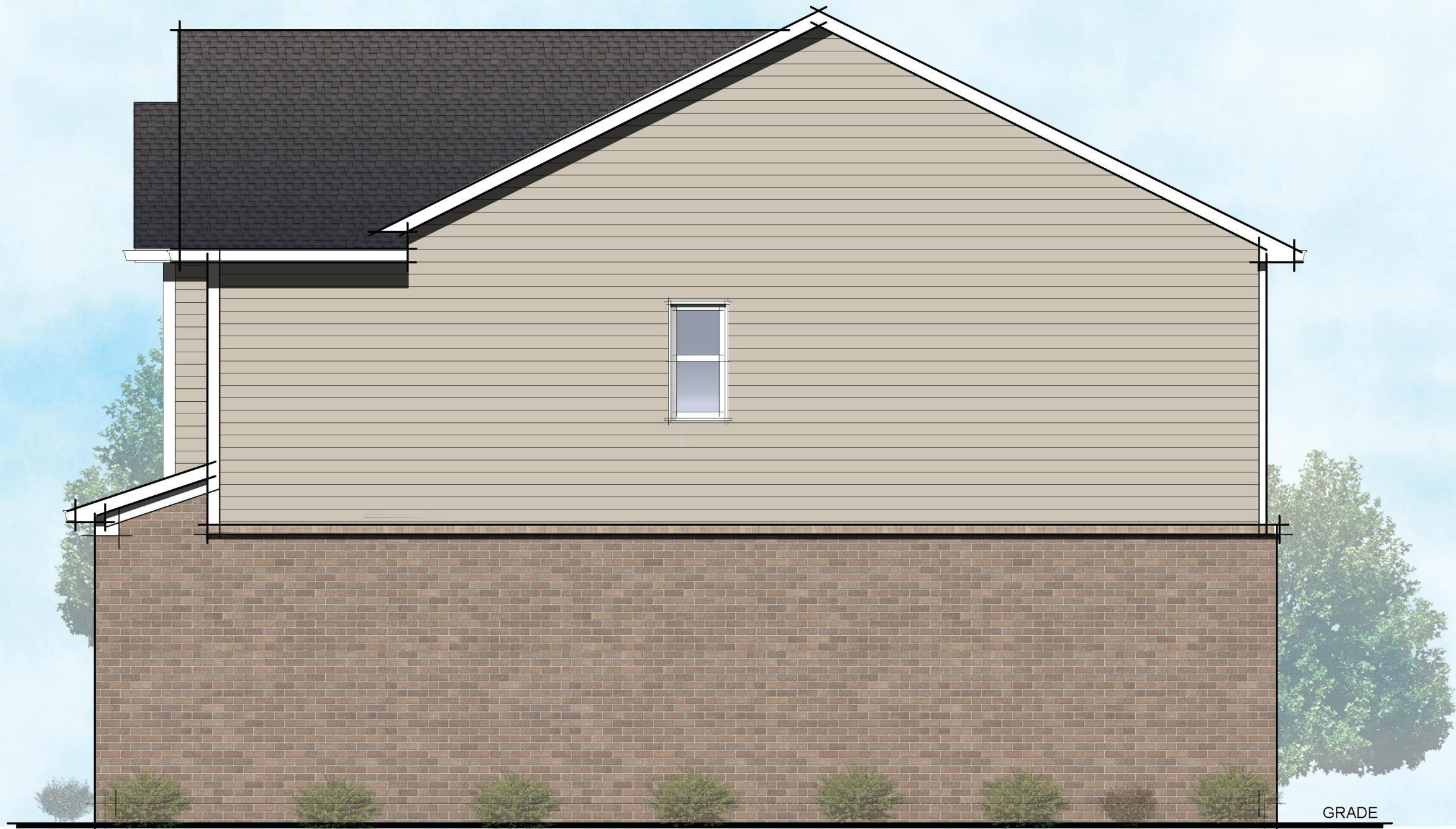
TYPICAL RIGHT SIDE ELEVATION ESSENTIAL SERIES 6 SCALE: 1/4" = 1'-0"
