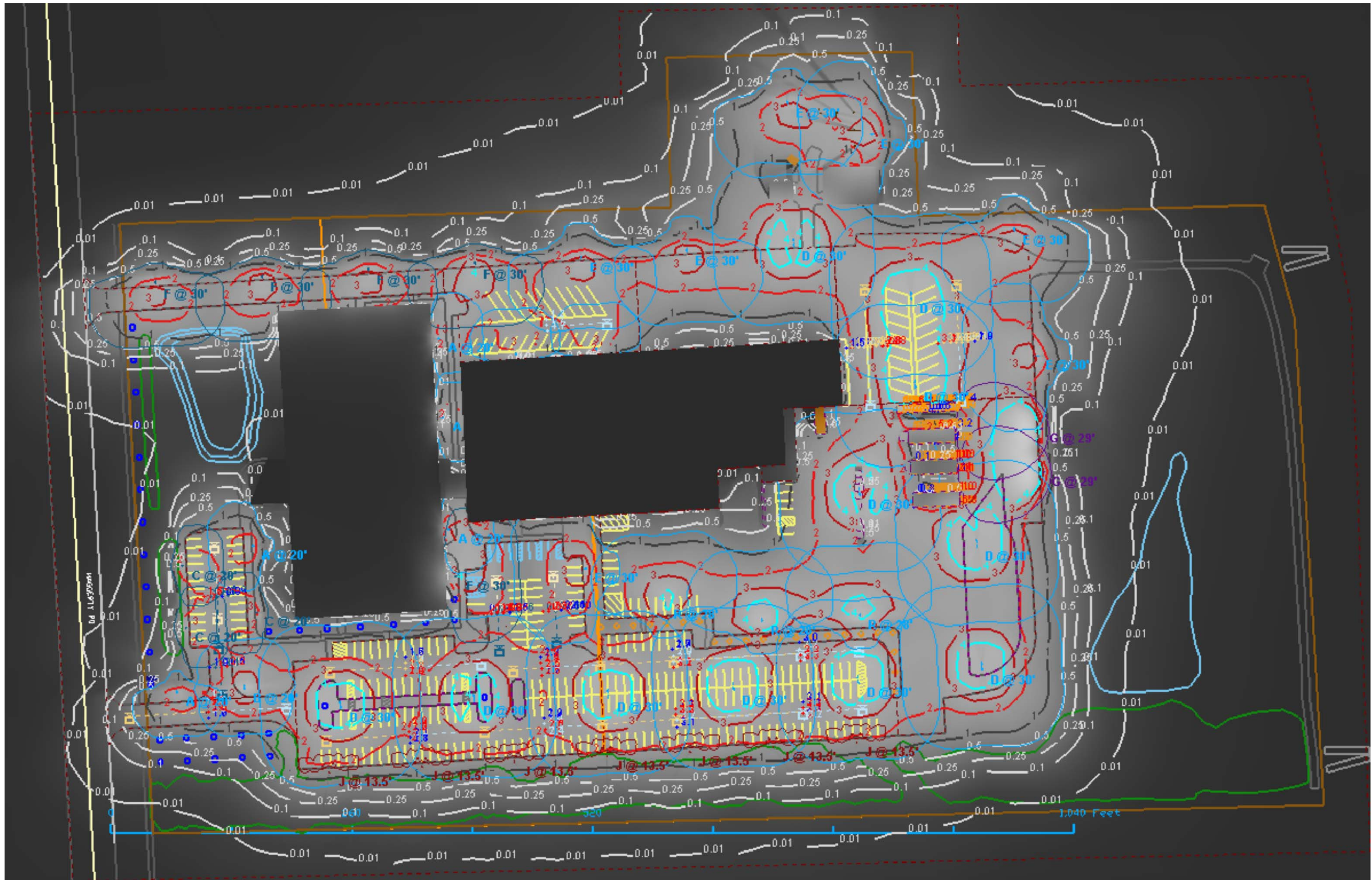
Site Plan Rendered with Lighting System Contours View #1
