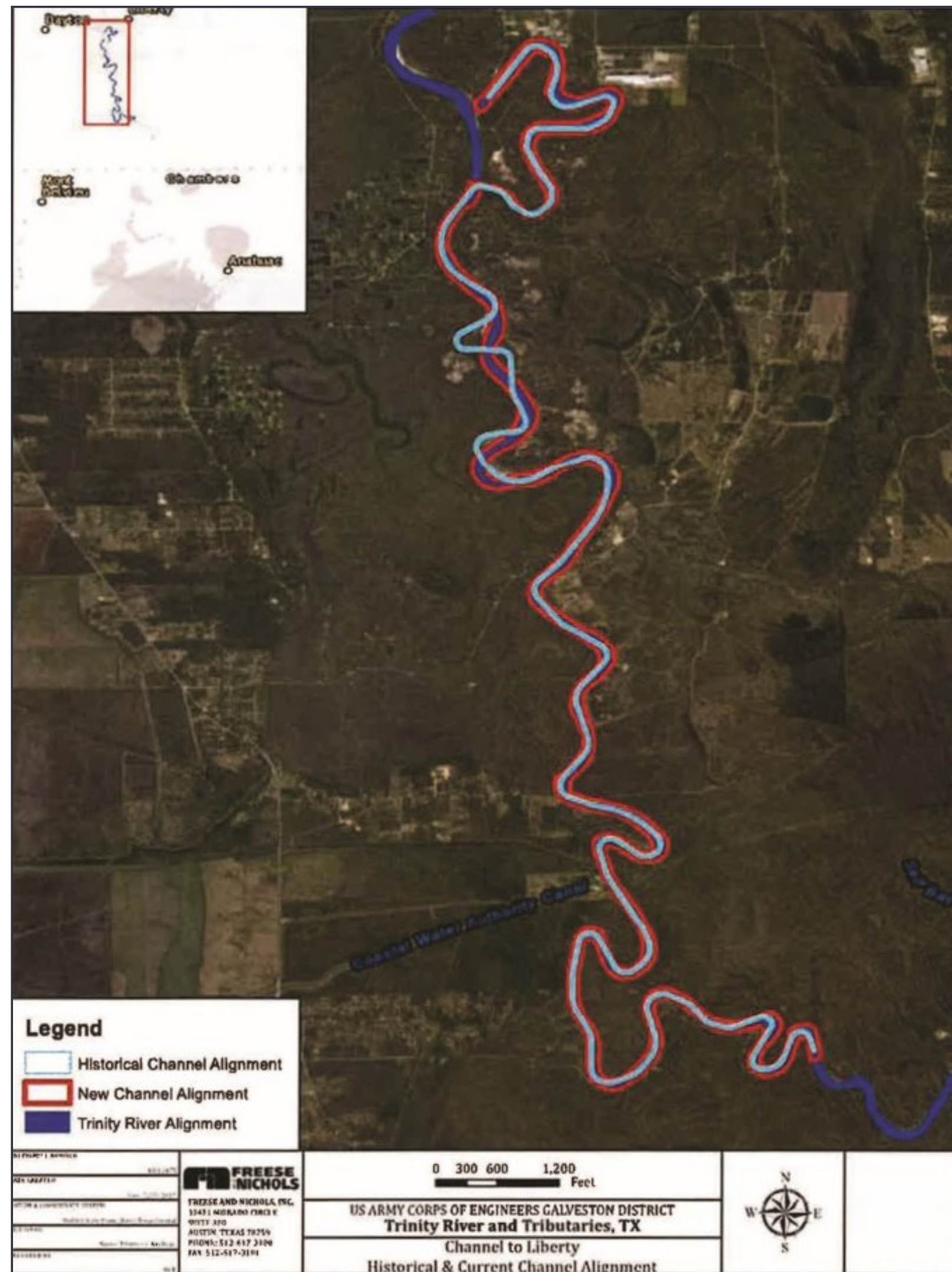
Figure 86. Channel to Liberty Overlay Historic and New Channel Maintenance Centerline (USACE 2017)
