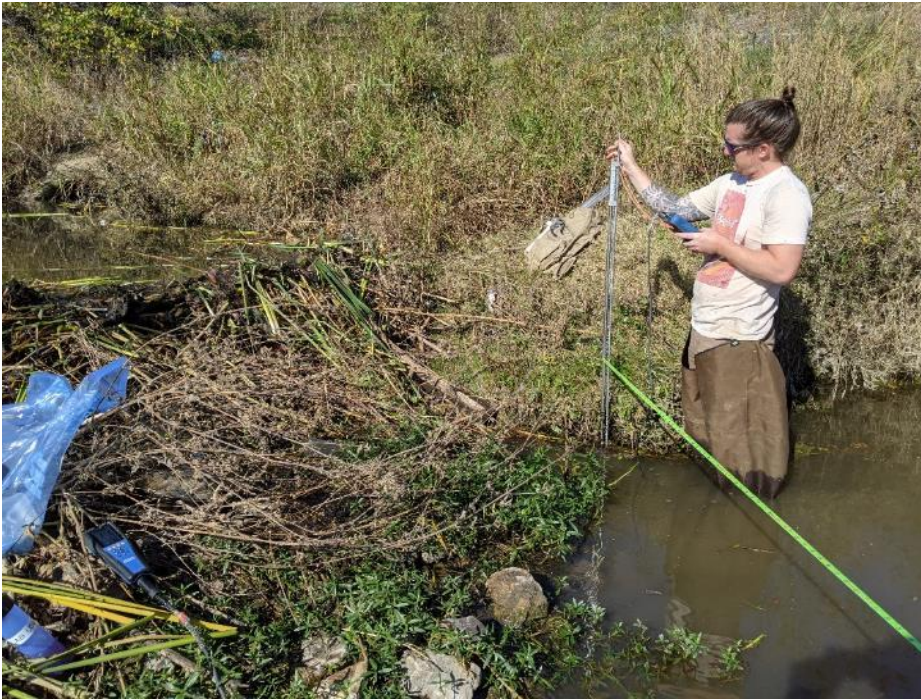
Figure 5-1 TRA staff conducting stream flow measurement on Bowman Branch in the JPL watershed
