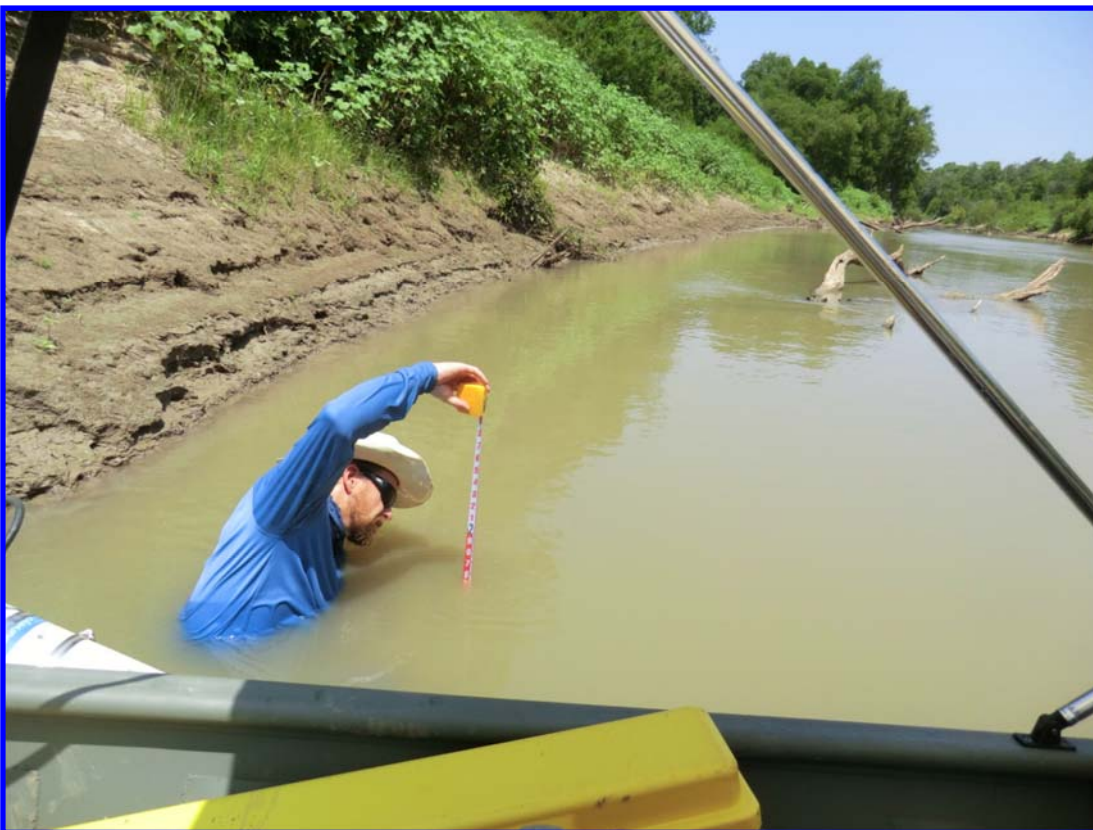
Fig. 8b. TRA field staff member collecting stage height during a pressure transducer installation in the Trinity River near Oakwood.
