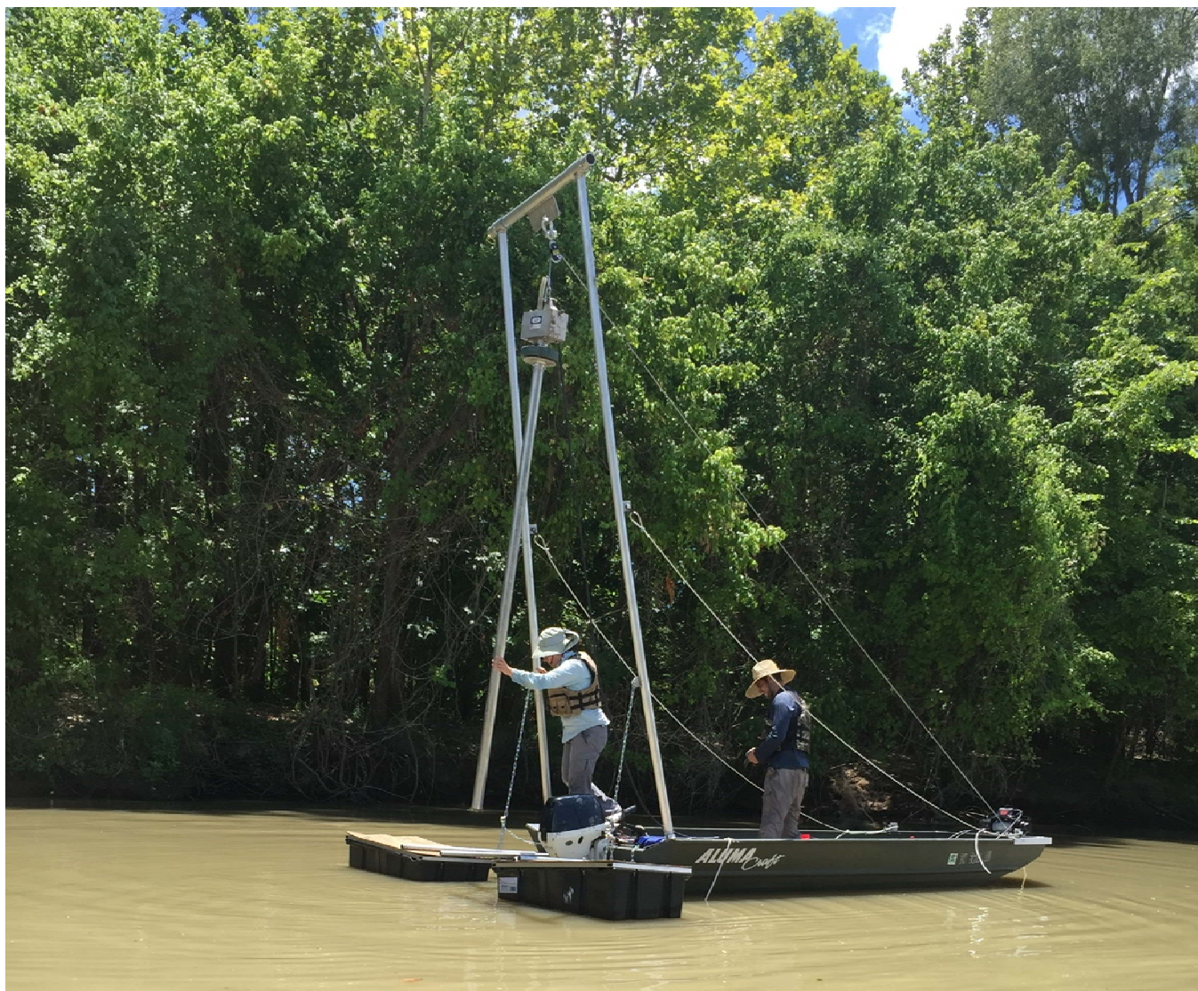
Figure 7: SDI VibeCore system being used by Arroyo Environmental Consultants, LLC in Lake Livingston at site 10914.
