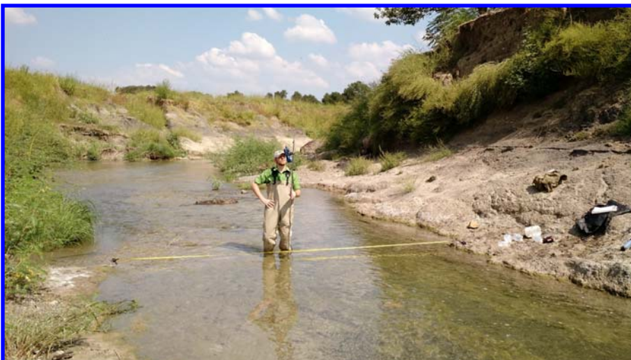
Fig. 4c. TRA Staff Measuring discharge at Ten Mile Creek
