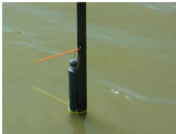
Figure 3-10. Overnight deployment of sonde at station 1
