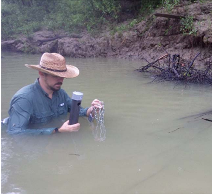
Figure 3. TRA staff deploying water quality sonde on the middle Trinity River near US Hwy 287.
