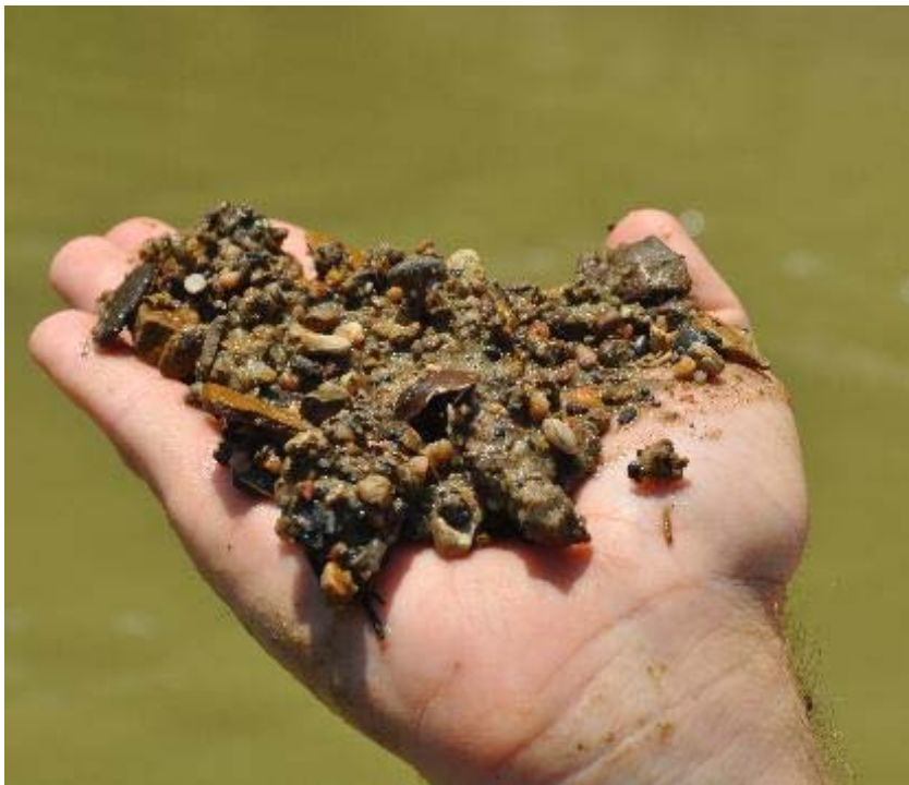
Figure 4. Sediment collected at one site along the middle Trinity River and categorized as small gravel according to the modified Wentworth Substrate Scale.
