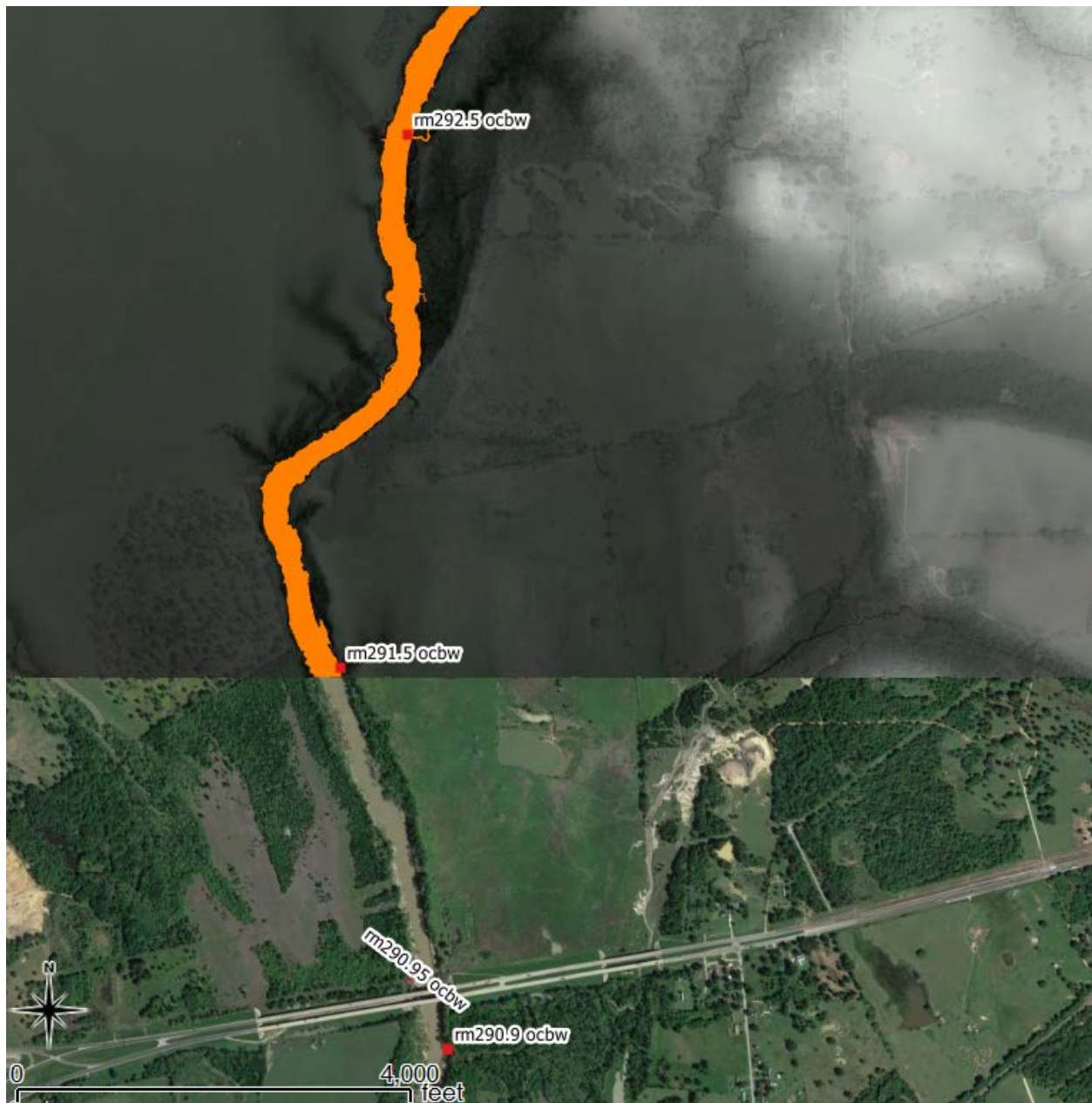
Figure 30. Segment C3 downstream of 080295 4 of 4 - Observed inundation and connectivity areas over the RAS 13400 cfs inundation map (orange). Note: Numbers represent approximate river mile.
