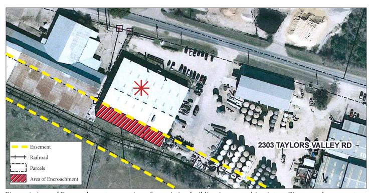
Figure 4: Area of Encroachment - a portion of an existing building is encroaching into a City owned easement.
