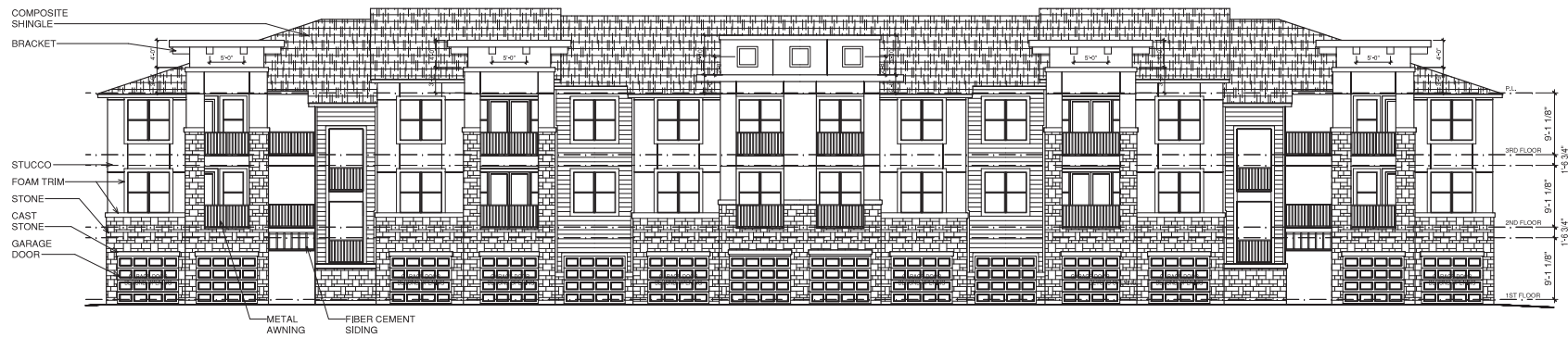
1 BUILDING 'A' FRONT ELEVATION (SOUTH) SCALE 1/8" = 1'-0"
