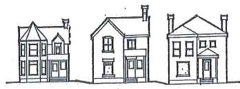
Avoid—Introducing incompatible facade patterns that upset the rhythm of openings established in surrounding structures. Glass walls and window and door shapes and locations shown in the example are disrespectful to the adjoining buildings.
