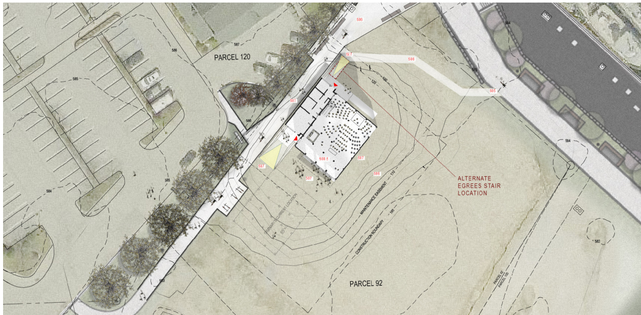
Image 8: Site Plan showing Granary's Current Location, Proposed (Original) Location, 120'x160' Construction Boundary and 100' x 110' Maintenance Easement (note that grading is preliminary)
