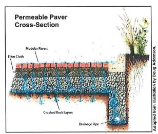
**Purpose:** By infiltrating precipitation, pervious pavement reduces stormwater runoff flow rate, volume, and temperature, and filters pollutants that would otherwise run into lakes, rivers, and wetlands. Pervious pavement also helps recharge groundwater and maintain stream base flows.
