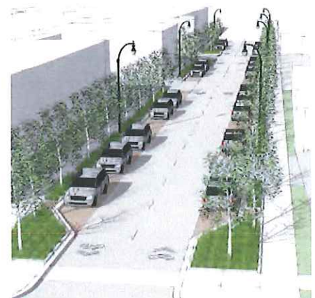
Green infrastructure concept for reconstructed downtown street using permeable parking bay paving, tree trenches and shared bike lanes.
