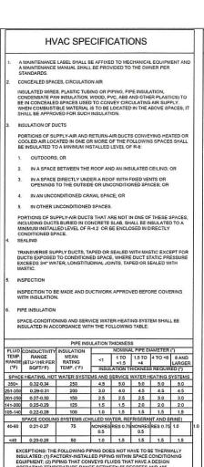
TING TEMPERATURE RANGE BETWEEN 55 DEGREES AND 105 DEGREES FAHRENHEIT; (3) GAS PIPING; (4) COLD DOMESTIC WATER PIPING (5) DRAINS, VENTS, AND WASTE PIPING
