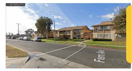
Lastly, a new curb ramp will be added on the westside of Fern Avenue at Palais Road to aid residents in crossing at the existing intersection. A mockup of the location is located below. The white "striping" shown in the photos is just to emphasize that the new curb ramp is supposed to line up with the existing curb ramp on the opposite SE corner of Fern and Palais. There will be no striping installed.
