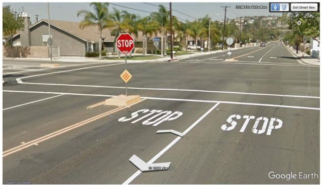
Sample of what the small median and new stop sign would look like. The Traffic Engineer proposes to add LED lights around the stop sign.
