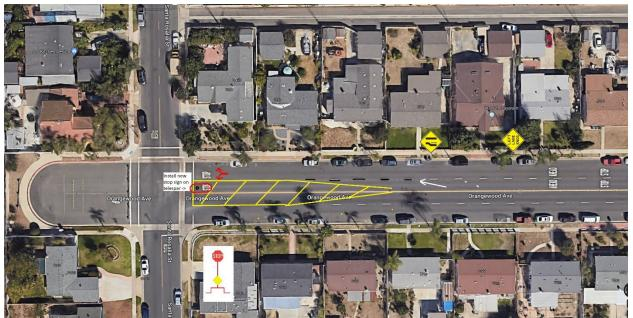
Proposed signing and striping plan for traffic safety improvements. Red oval outline indicates size of small median island to accommodate proposed center-of-road mounted stop sign.
