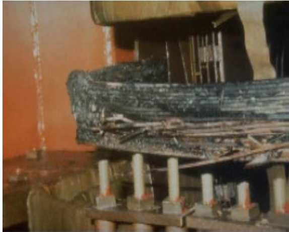
Permanent damage to the Salem New Jersey Nuclear Plant GSU Transformer caused by the severe geomagnetic storm of March 13, 1989 (Credit: PSE&G)
