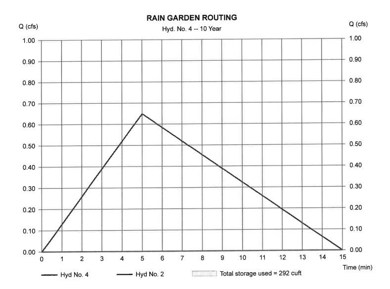
Hydraflow Hydrographs by Intelisolve v9.1
