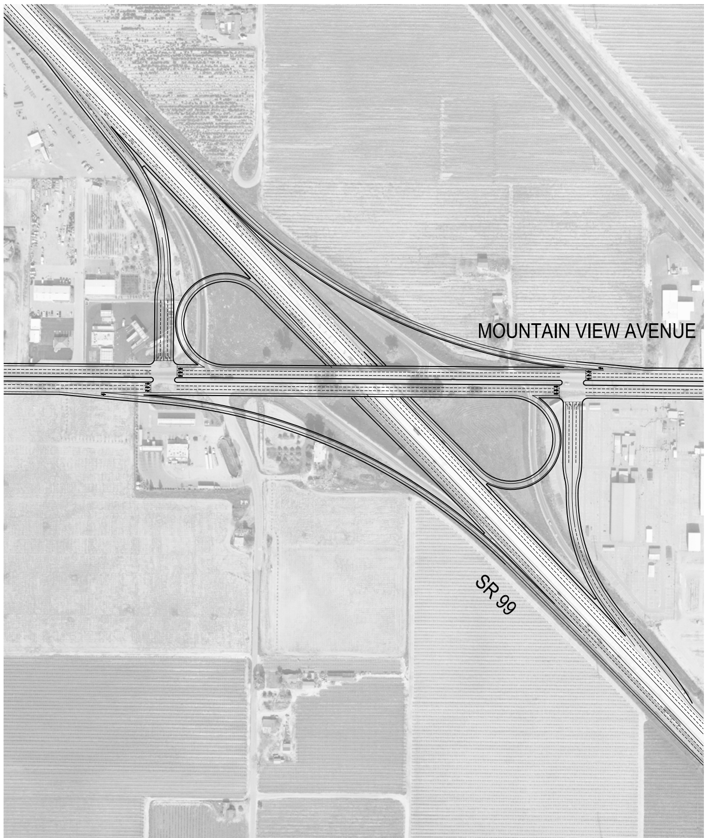
CONCEPTUAL INTERCHANGE LAYOUT MOUNTAIN VIEW AVENUE AND STATE ROUTE 99 GENERAL PLAN UPDATE Selma, California
