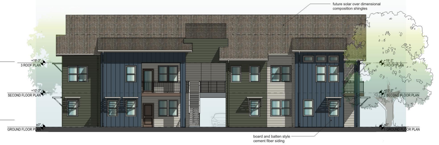
3 FRONT ELEVATION BLDG A SCHEME 1 SCALE: 1/8" = 1'-0"
