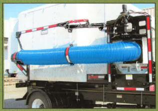
ODB's 3 axis boom allows smooth, precise movement of the suction hose to the leaf pile. Combining two hydraulic cylinders for the up/down and in/out movements, plus a planetary, wheel drive hydraulic motor for the left/right movement
