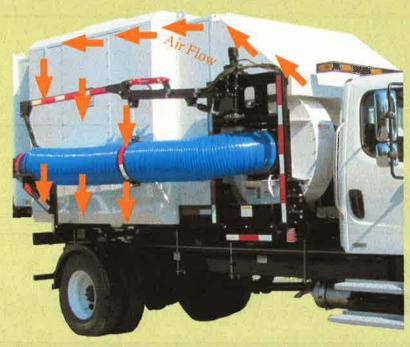
Air is vented through heavy duty mesh screens mounted in the top of the box and then directed to the sides by all steel duct work and is exhausted on to the ground.
