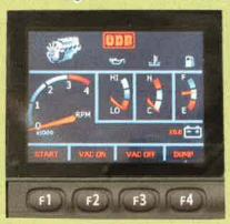
IOAN controls allows for a "user friendly" access to all controls and features. Simple function keys and full color graphics allow the operator to easily use all the features of the unit.
