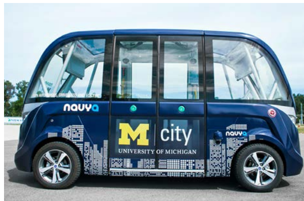
Autonomous shuttle bus at the MCity testing grounds in Ann Arbor. Source: New York Times
