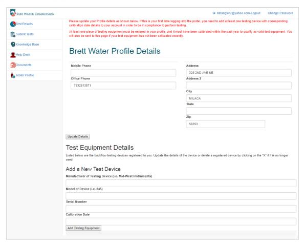
Each Tester must register a test device used for Backflow Prevention testing. The Manufacturer, Model and Serial Number of the test equipment must be populated. Plus, the Calibration Date of the device must be entered as well. Once this information is entered, click the **Add Testing Equipment** button.
