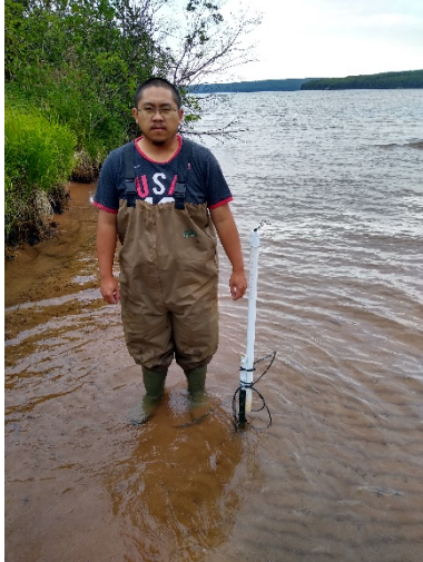
TNR technician next to an antenna at the Raspberry River site. The t-post was above the technician's head before getting buried under several feet of sand.
