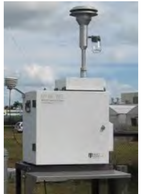
Photo 1. An example of a 2025i Thermo-Partisol Sequential Air Sampler.
