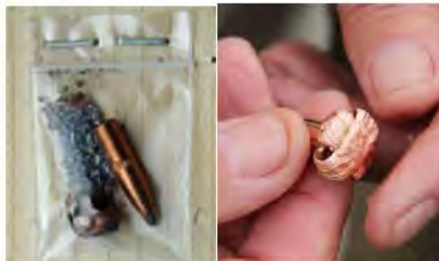
On left: Lead rifle bullet with fragments produced. On right: Ammo made out of copper has no fragments
