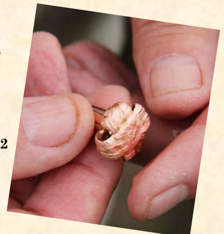
On left: Lead rifle bullet with fragments produced. On right: Ammo made out of copper has no fragments
