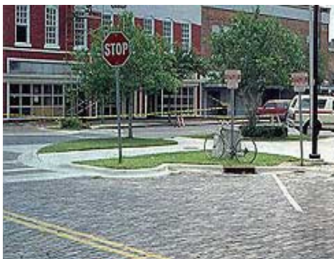
Textured pavement in Gainesville, FL: textured pavement combined with diagonal parking.
