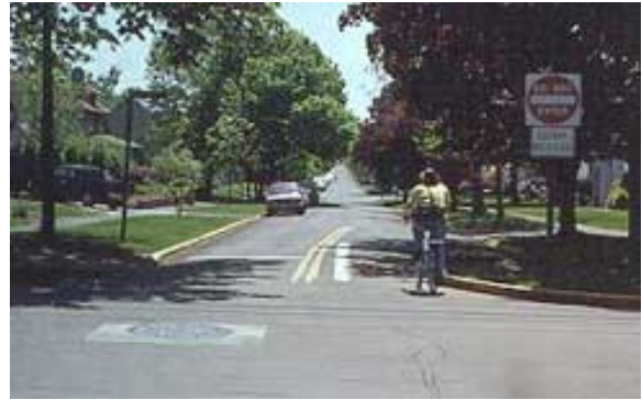
Half-street closure, Eugene, OR: blocks entry in one Direction by cars but allows access for bikes
