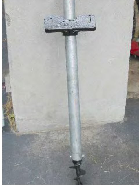
Figure 7 – Pipe with auger and dock fitting attached.
