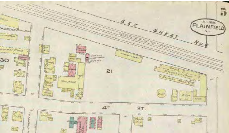
These two 1886 Sanborn Fire Insurance Map Plainfield sheet sections 33 show the station as a masonry structure with a perimeter wood roof assembly. The station had the main passenger area in the center flanked by open passageways on each side, a large smoking room was to the east, and baggage room and freight office was to the west. Note that street in front of the station runs straight in line. To the south of the tracks a frame freight depot stood in an open area, logically facilitating wagon traffic.
