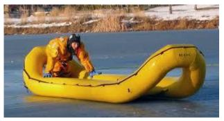
caught in swift water, or have fallen through thin ice. This device can be inflated in under a minute and be quickly deployed by two firefighters. It is designed so that victims can be pulled up onto its deck from either of the two openings in the craft's front or back.
