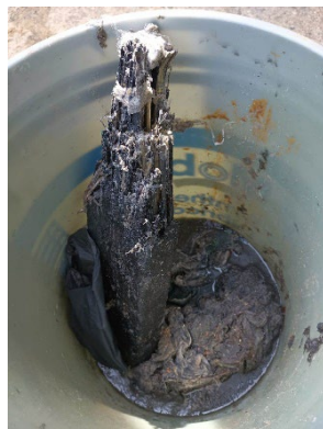
Piece of 2 x 4 board removed from pump at PS #18
