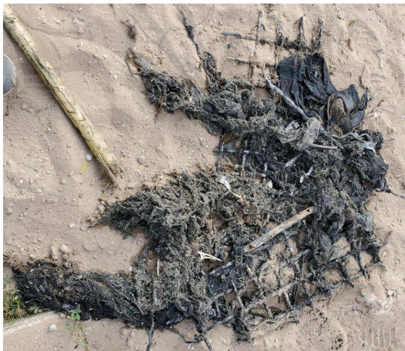
Metal debris and rags removed from Pump Station #4 wetwell
