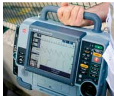
Dual-mode LCD screen with SunVue display
