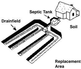
The typical septic tank is a large buried rectangular, or cylindrical container made of concrete, fiberglass or polyethylene. Wastewater from your toilet, bath, kitchen, laundry, etc., flows into the tank. Heavy solids settle to the bottom where bacterial action partially decomposes them to digested sludge and gases. Most of the lighter solids, such as fats and grease, rise to the top and form a scum layer.
