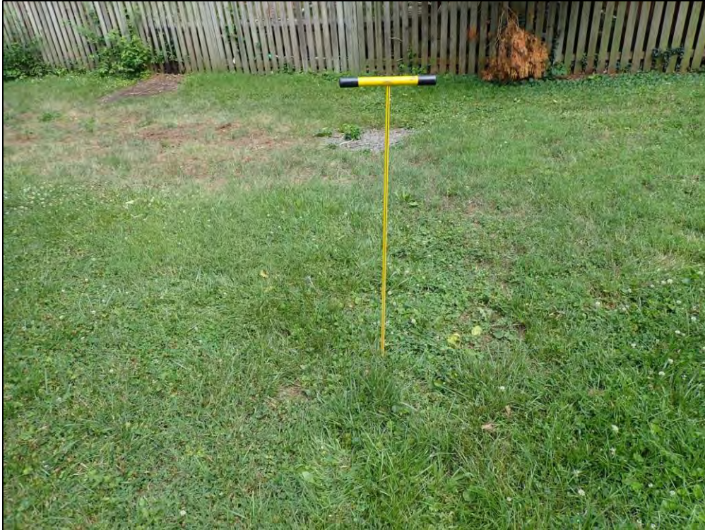
4811: Gravel detected approximately 3" beneath the surface. Evidence of clogging (Immediate Repair Needed).
