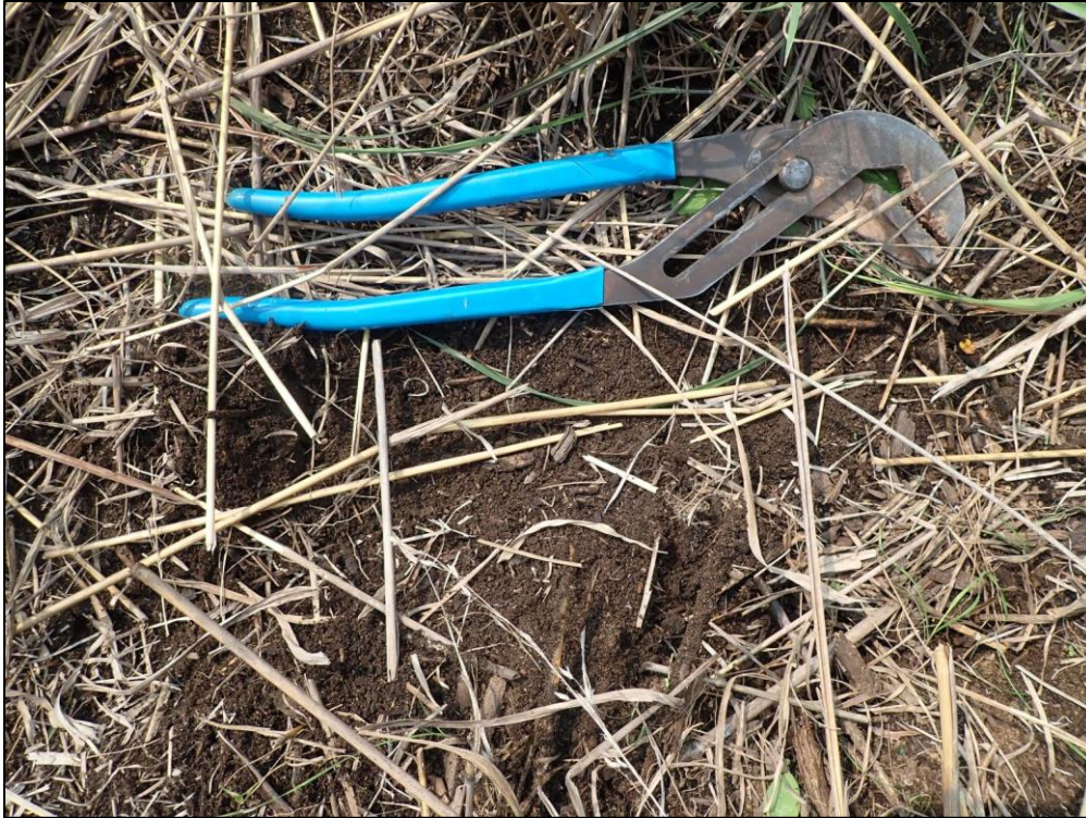
5006: Close-up of the ponding area showing 0" of mulch. Mulch layer is less than 2" deep or is otherwise in poor condition (Routine Maintenance Needed).
