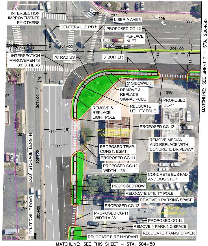
**DRAFT** THIS CONCEPTUAL PLAN WAS PRODUCED FOR DISCUSSION PURPOSES ONLY. PROP FULL DEPTH ASPHALT PAVEMENT PROP CONCRETE (SIDEWALK/ MED) PROP GRASS MEDIAN/ BUFFER PROP MILL AND OVERLAY PROP CURB & GUTTER
